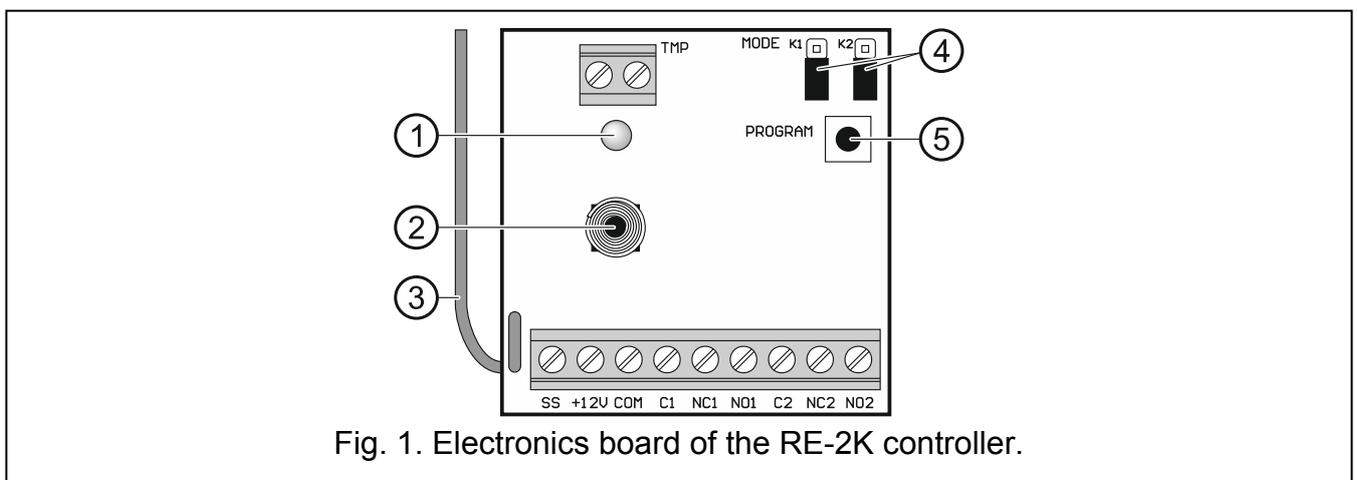
Fig. 1. Electronics board of the RE-2K controller.
