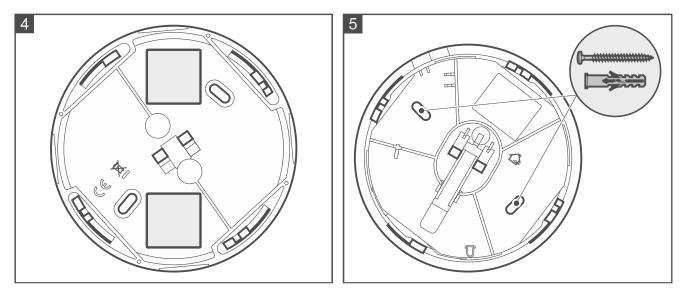
12. Replace the detector cover and lock it with a screw. The screw is provided in a bag together with the wall plugs and screws for mounting.
