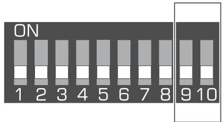
Fig. 2. Switches defining the controller operating mode.
