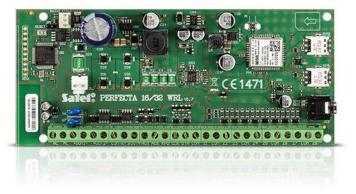
sounds from the protected premises). Two nano-SIM cards are supported to ensure continuity of communication: if any problems occur with the first operator range, the second card is automatically selected.
